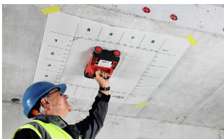
c) Scanning for ferrous and non-ferrous objects
