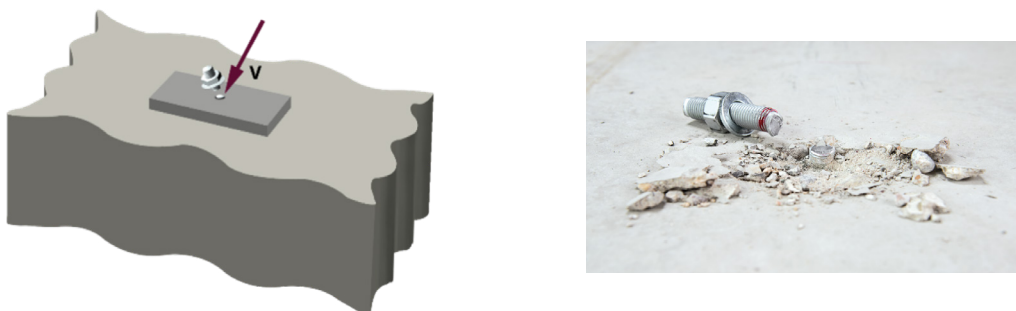
a) Failure without lever arm
