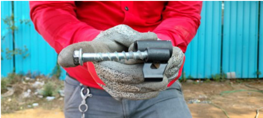
b) Hilti anchor with re-usable gauge
